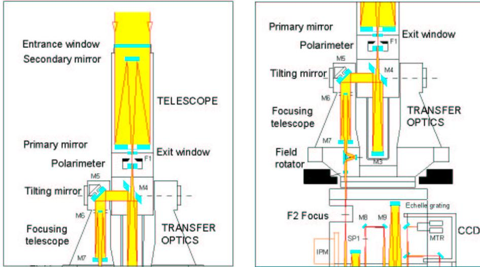
Figure 1. Optical schemes of (left) the telescope and polarimeter, and (right) the F1–F2 transfer optics.
