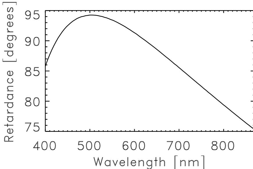
Figure 2. Retardance vs. wavelength of the quarter wave plates used in the polarimeter. Those achromatic QWPs are made of 2 crossed elementary thin crystalline plates of  $\text{MgF}_2$  and quartz, with anti-reflection coating (manufactured by *Optique J. Fichou*, France).
